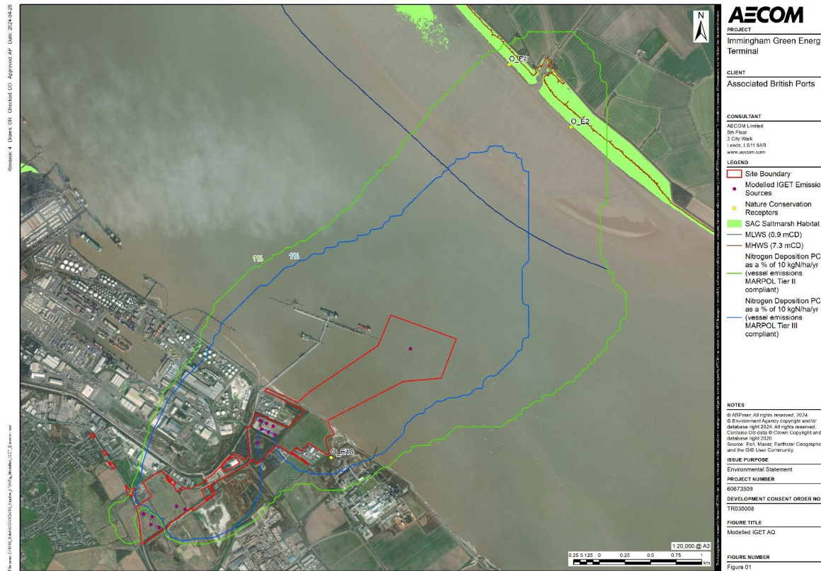
Plate 3: Isopelth Diagram (operational N deposition assuming a precautionary 10 kgN/ha/yr as the suitable critical load)
